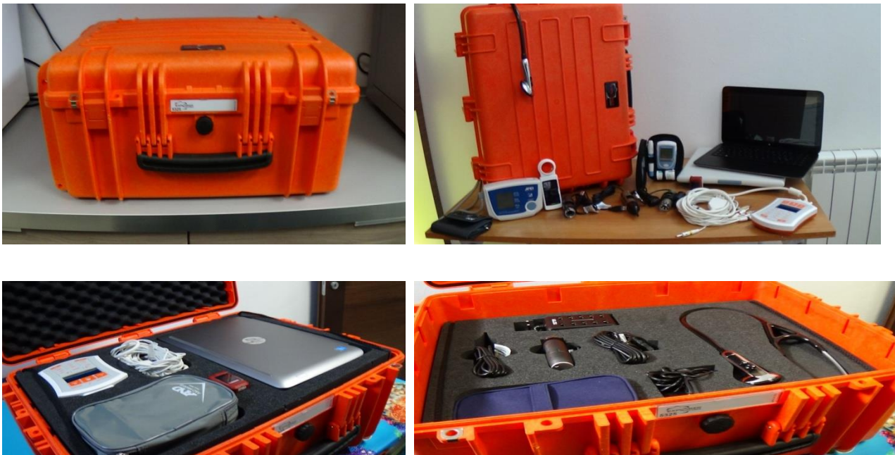
Figure 11: Telemedicine case already installed or being installed in 2015 on board of 50 ships belonging to the France company CMA Ships in Marseille. The case contains an artificial intelligence system for helping to prepare a more precise request of medical advice (24) and the telemedical devices listed below: Infrared thermometer, High quality photocamera, Electronic phonendoscope, Blood pressure monitor, 12 derivations ECG, Spirometer and SPO2, Glucometer
